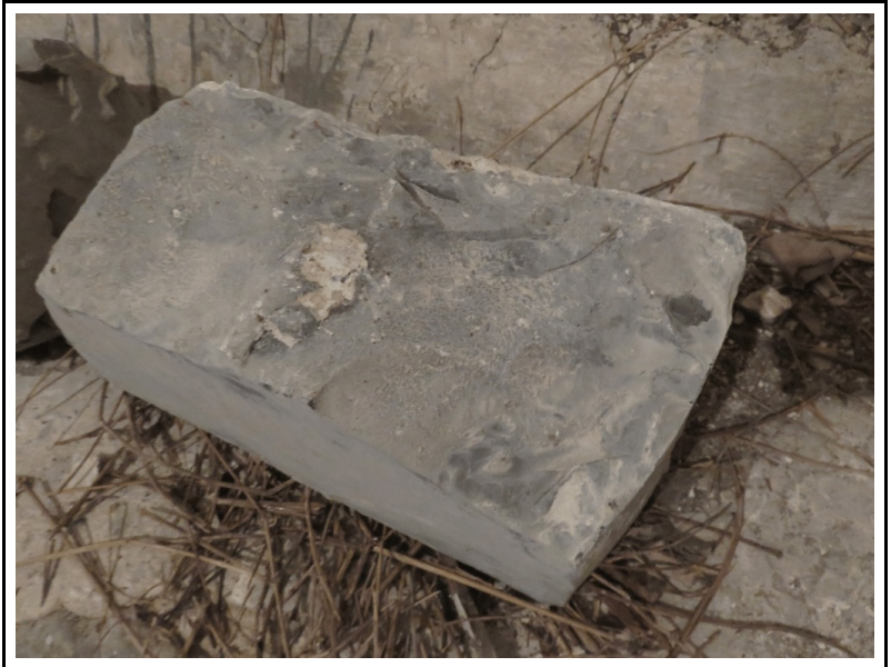
Photo 2: This stone unit, which was apparently removed from the interior masonry, appears to be a very dense, tough but brittle limestone.
